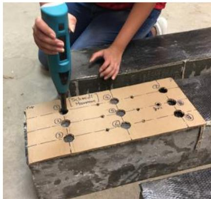
Figure 7. Schmidt Hammer Test
