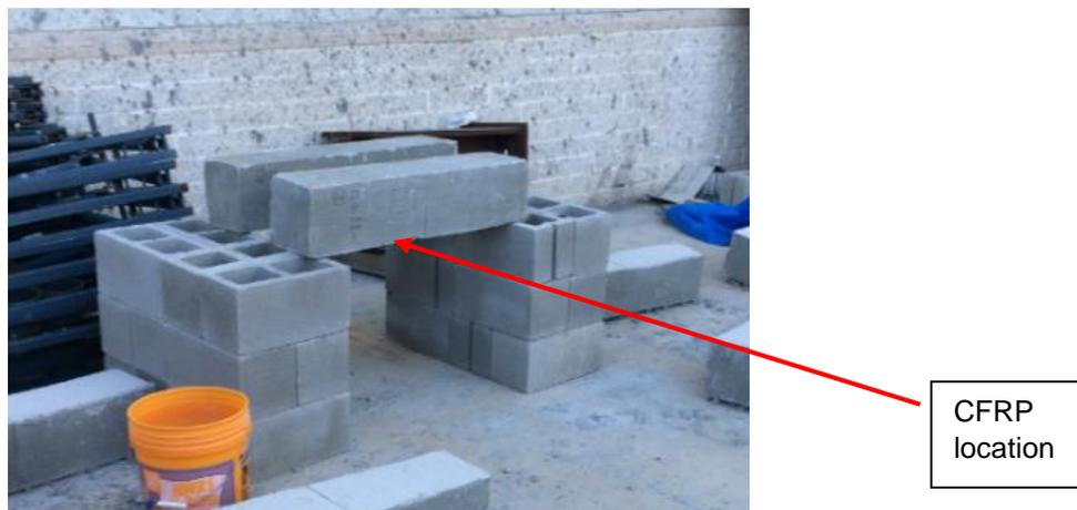
**Figure 6.** Setup for Upward application of CFRP
