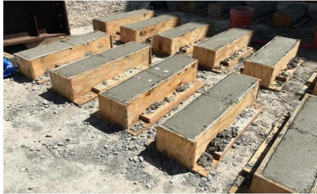
**Figure 2.** Concrete Beam Specimens
