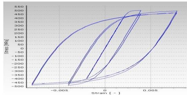
Figure 5. Cyclic behaviour model of steel [50]
