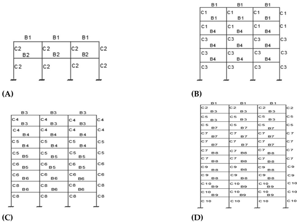
Figure 4. Design sections of steel moment resisting frames (A, B, C and D represented frames with variable height)
