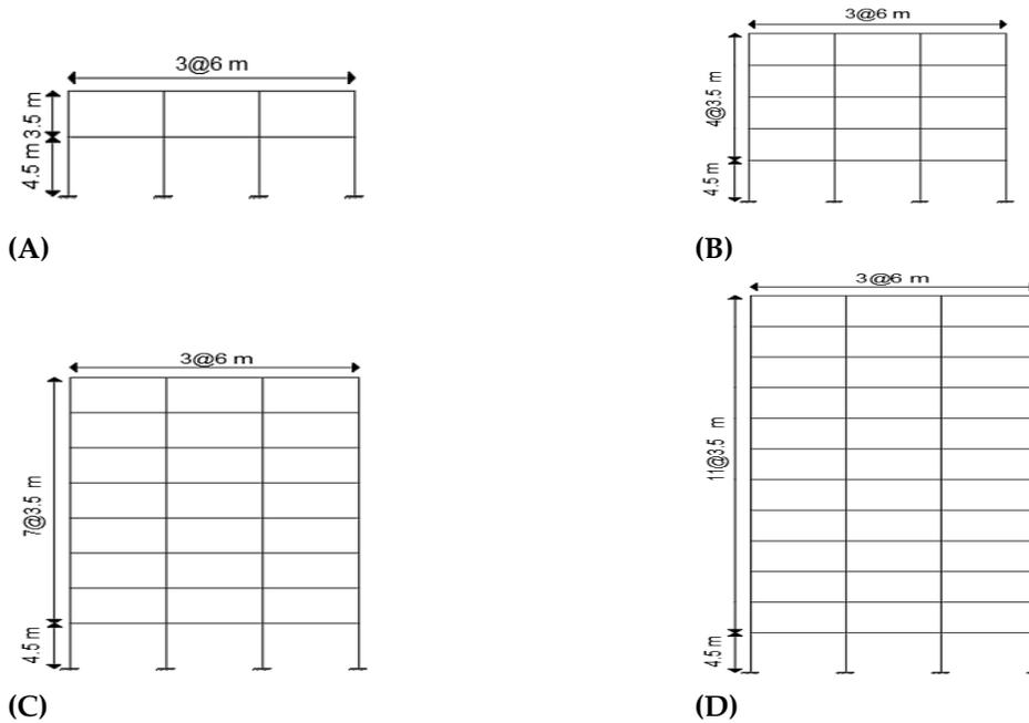
Figure 3. Geometrical specification of steel moment resisting frames (A, B, C and D represented frames with variable height)
