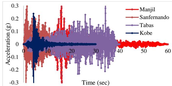
Figure 7. Studied accelograms scaled to base design acceleration
