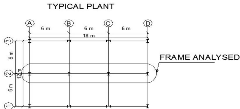
**Figure 2.** Typical plant of steel moment resisting frames [46]
