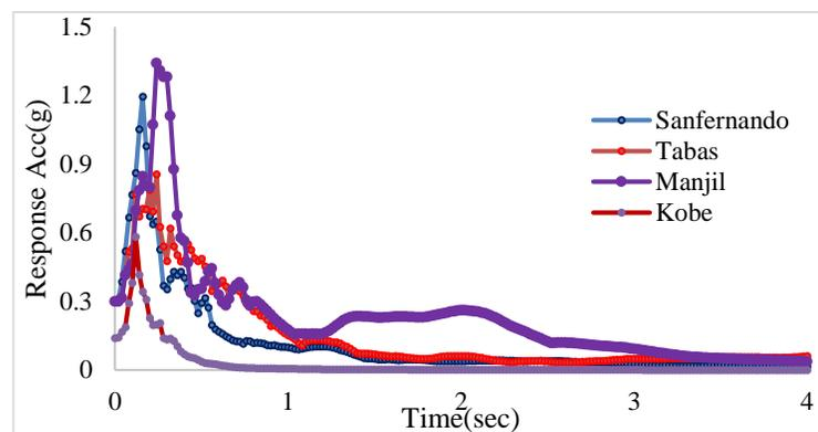
Figure 8. Elastic acceleration response spectrum scaled to base design acceleration with 5% damping
